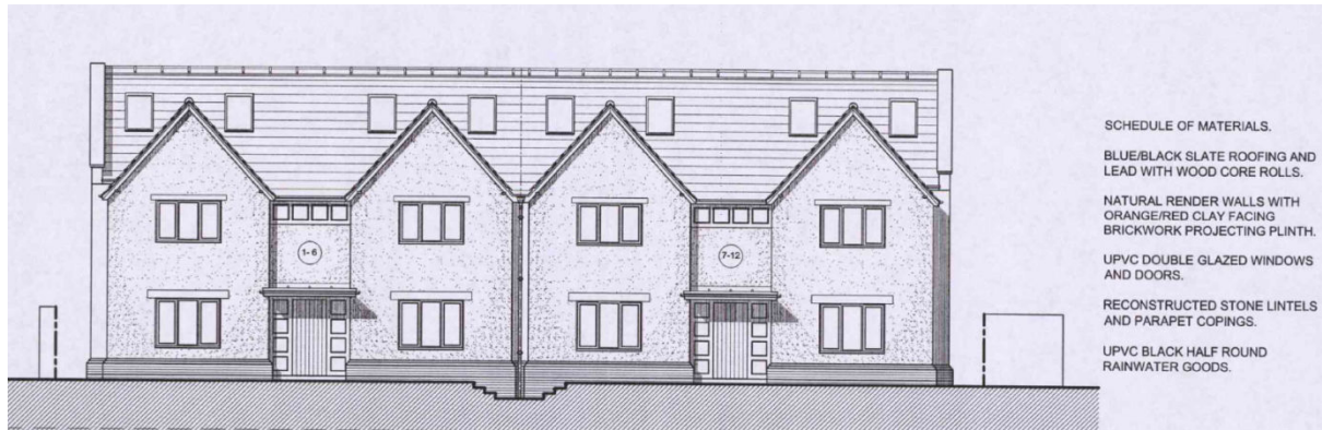
Front elevation of approved scheme
